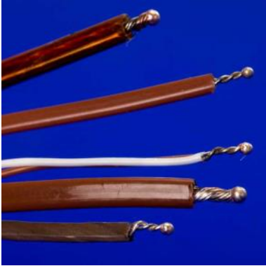
Pre-cut Validation Thermocouples
