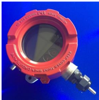
Field Mounted Transmitter
