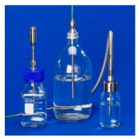
GL45-1 Bottle Cap Gland for Thermocouple
