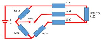
In this configuration the detector lead wires L1 and L3 are connected to the opposite sides of the bridge, effectively compensating for each other, with the third wire L2 supplying power to the bridge.
