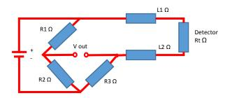
Where the lead lengths are short, and where they are exposed to the same temperature as the detector, then in theory this can be accounted for.
